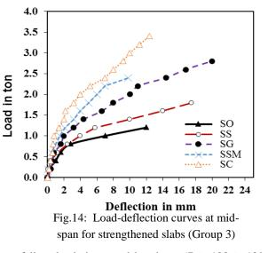
failure loads increased by about 67%, 108%, 129% and 170%, respectively.
