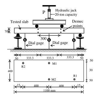
Fig. 3: Test setup and instrumentation
