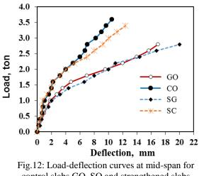
control slabs GO, SO and strengthened slabs SG and SC
