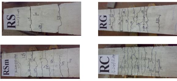
Fig.17: Crack patterns for repaired slabs (Group 2)
