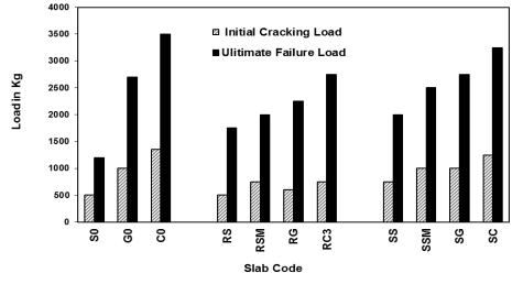
Fig.15: Comparison between cracking and ultimate loads
