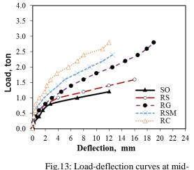
span for repaired slabs (Group 2)
