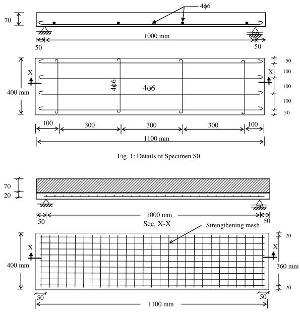
Fig. 2: Details of strengthening for specimens SSM, SG and SC
