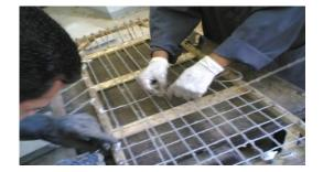
Fig.7: Intertwined GFRP roving submerged in epoxy
